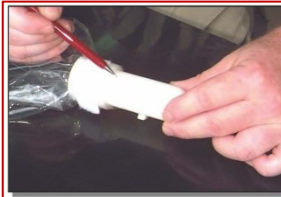
Figure 11-- Pressure equalization hole
