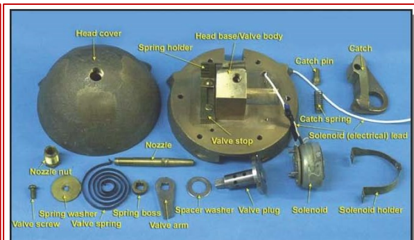
Figure 6. US P-61-A1 Head (disassembled)
